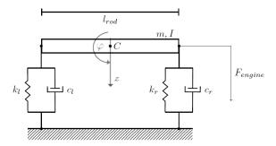
Analysis of the scheme allows to claim its number of degrees of freedom which is 2
